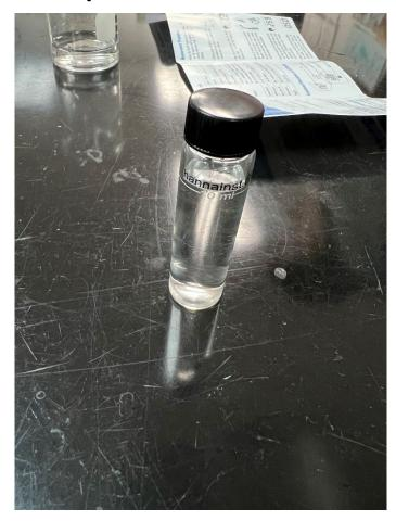
Step 3: Wipe off the cuvette. Make sure there are no droplets on the outside of the cuvette
