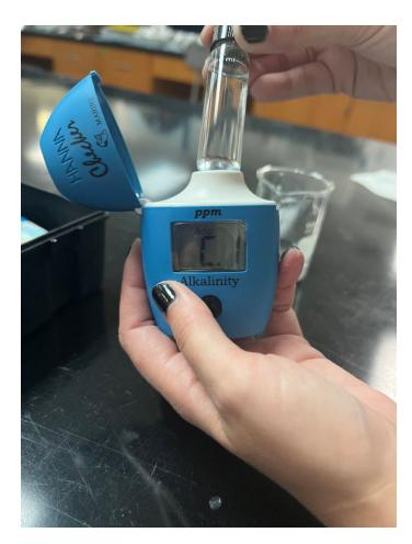
**Step 5**: **Tap** the on/off button When the display shows "ADD", "C.2", with "Press" blinking, the checker is zeroed
