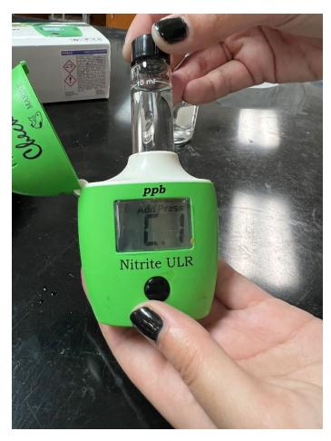
Step 5: Press the On/Off button. When the display shows "ADD", C2", with "Press" blinking, the
