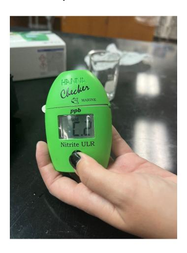
Step 9: **Press** and **HOLD** (for about 3 seconds) the on/off button. Release when the display shows a countdown. This countdown represents the checker reading the sample.
