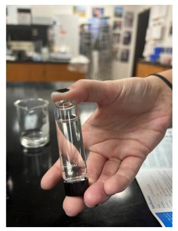
**Step 7**: Use 1 ml syringe and add exactly 1 ml of HI755S Marine Alkalinity reagent to the sample. **Note: 1 ml is at the bottom of the plunger**
