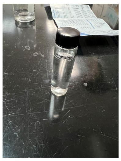
Step 3: Wipe off the cuvette. Make sure there are no droplets on the outside of the cuvette
