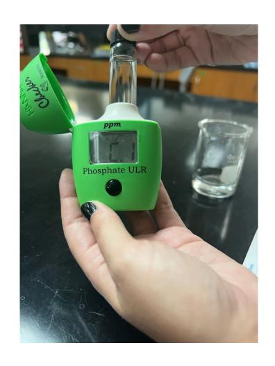
**Step 5**: **Press (tap)** the on/off button. When the display shows "ADD", "C.2", with "Press" blinking, the checker is zeroed
