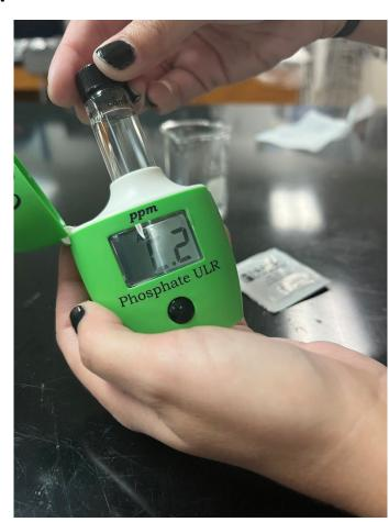
**Step 9**: **Press** and **HOLD** (for about 3 seconds) the on/off button. Release when the display shows a countdown. This countdown represents the checker
