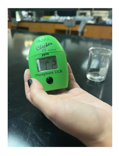
**Step 6**: Remove the cuvette, unscrew the cap and add the content of one packet of **HI774-0**
