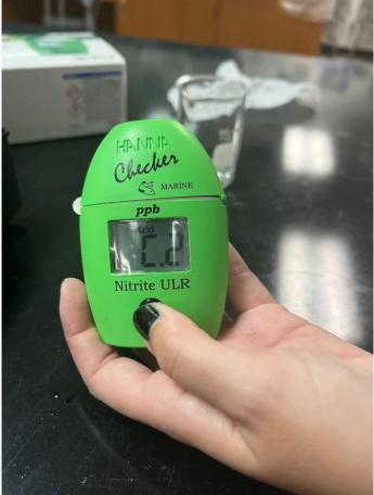
Step 6: Remove the cuvette, unscrew the cap and add the content of one packet of **HI764-0 Nitrite** Ultra Low Range reagent
