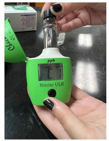
Step 5: Press the On/Off button. When the display shows "ADD", C2", with "Press" blinking, the checker is zero
