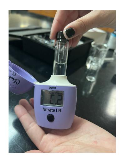
Step 18: Press and HOLD (for about 3 seconds) the on/off button. Release when the display shows a count down. This countdown represents the
