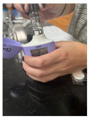
Step 14: **Press (tap)** the on/off button. When the display shows "ADD", "C2", with "Press" blinking the checker is zero
