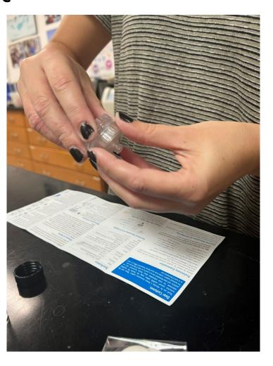
Step 8: Attach the filter holder assembly to the 10 ml syringe
